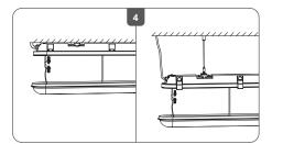
4. Connect the safety rope and Connect male/female DC connectors, Check all connections are sound and properly insulated, and fit the tray back in the casing
