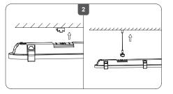
2. Position and fix base using the pre-fixed mounting brackets / suspension kits.
