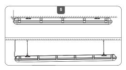
5. Re-fit the diffuser to the base and secure all the clips.
